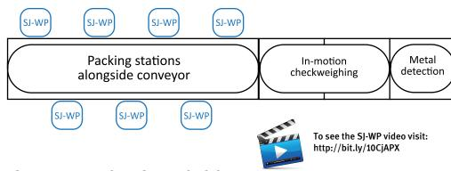
The SJ-WP is the start of a total solution for weighing and packing. Use the SJ-WP to load containers prior to metal detection and wrapping. Accurate and fast enough for packing product lines; tough, portable and battery powered to pack even in the field.
