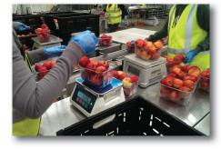
Fruit baskets packed and weighed on the SJ-15WP prior to in-motion checkweighing and metal detection.
