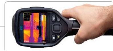
Auto-Orientation Keeps Diagnostics Overlays Upright
