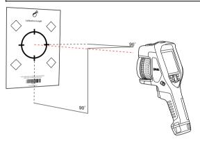
In the camera, align the thermal and visual images (indicated by the two squares in the image below), using the touchscreen arrows. The lens–camera combination is now calibrated.
