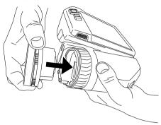
6. Rotate the inner ring of the lens  $30^\circ$  clockwise. The lens makes a click when it locks in place.
