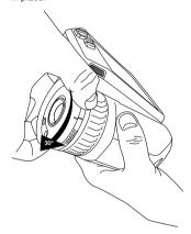
Make sure that the two index marks are aligned, indicating that the lens is locked in place.
