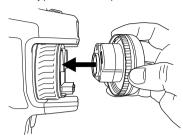
Rotate the inner ring of the lens 30° clockwise. The lens makes a click when it locks in place.
