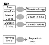
Save the logs as waveform data or as image files
