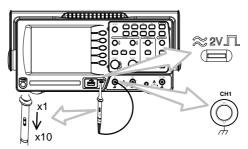
8. Press the Autoset key. A square waveform will appear in the center of the display. For details on Autoset, see page 45.
