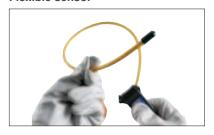
Traditional approach: attempts to snake flexible sensor around cable may lead to electric shock
