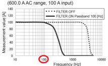
Turn off the filter function when performing measurement of power supply frequencies in excess of 100 Hz, for example on an aircraft or ship.
