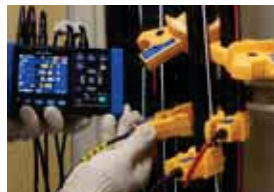
Measure on the outside of cables
