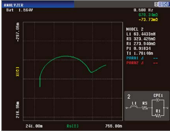
Cole - Cole plot screen (manganese battery)
