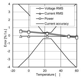
Fig. 14. Effects of Temperature (50 Hz)
