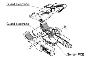
Fig. 8. Exploded View of the Sensor Assembly
