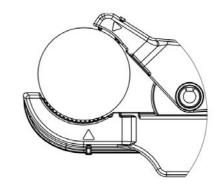
Fig. 7. When Clipping to a Cable With a Diameter of 30 mm
