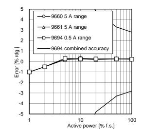
Fig. 12. Power Linearity Characteristics (50 Hz)
