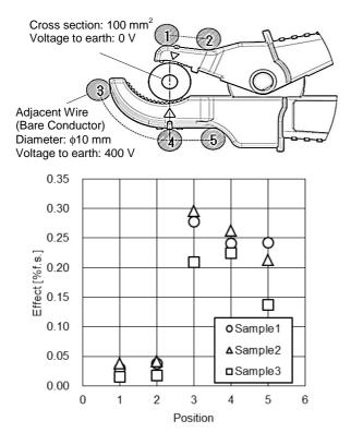
Fig. 15. Effects of Nearby Wires (50 Hz)
