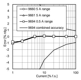
Fig. 11. Current Linearity Characteristics (50 Hz)
