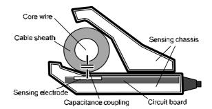
Fig. 1. PW9020 Electrode Design (Cross-sectional view)
