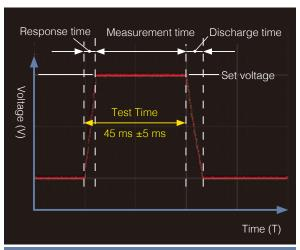
Applied Voltage Waveform at Fastest Test Time
