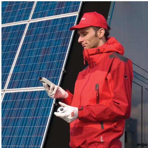
Figure 2 pyranometer in use with LI19 read-out unit
