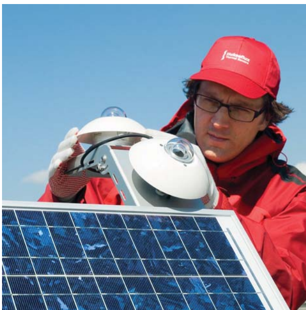
Figure 2 PV system performance monitoring pyranometers
