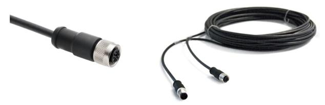
**Figure 0.7** On the left the SR30 cable with M12-A female connector on sensor end, pigtails of 0.15 m and conductors with ferrules. Its length is 5 metres standard and available in 10 and 20 metres too. On the right the optional Hukseflux extension cable with connector pairs, with male and female M12-A connectors, available in 20 metres
