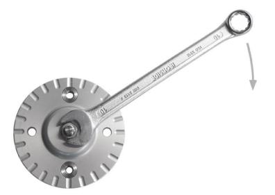
Figure 6.3.1.3 SR30 levelling mount seen from above: (un)locking with a 10 mm spanner
