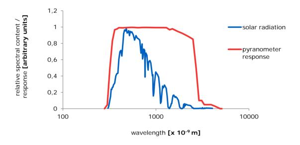
**Figure 2.0.2** Spectral response of the pyranometer compared to the solar spectrum. The pyranometer only cuts off a negligible part of the total solar spectrum.
