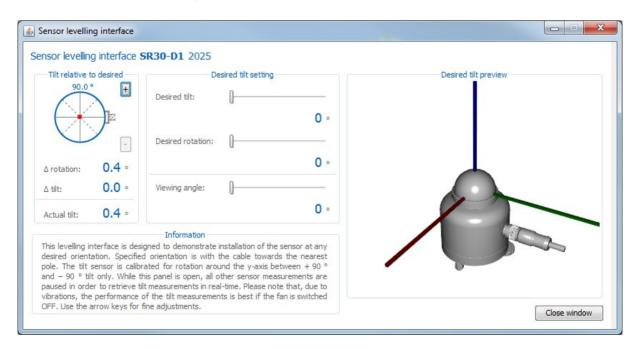
Figure 7.1.8.1 Sensor levelling interface in the Sensor Manager
