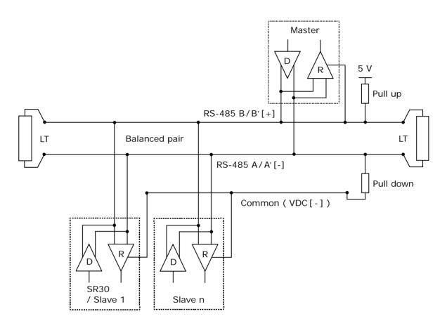
**Figure 6.7.1** Typical topology of a two-wire RS-485 network, figure adapted from: Modbus over serial line specification and implementation guide V1.02 (www.modbus.org). The power supply is not shown in this figure.
