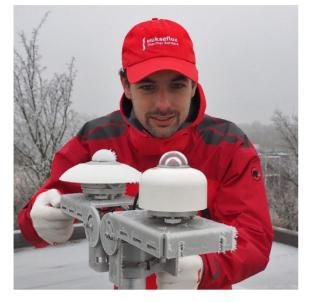
**Figure 0.2** Dew deposition and frost (as in the photo): clear difference between a non-heated pyranometer (back) and SR30 with  $RVH^{TM}$  technology (front )
