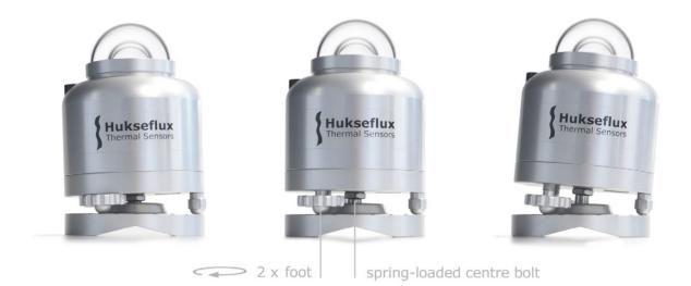
**Figure 6.3.1.5** *SR30* locked on its optional levelling mount: by fastening (on the left) or loosening (on the right) *SR30*'s two adjustable feet, *SR30* can be levelled, judging by the bubble level. *SR30*'s static foot remains fixed. In all cases, ensure the legs of SR30 fit into one of the small ledges of the levelling mount. Locking is in place, when the nut is turned all the way against the bottom plate of SR30
