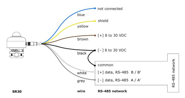
Figure 7.3.1 Connecting SR30 to a typical RS-485 network
