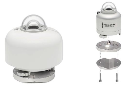
**Figure 0.5** Optional levelling mount (picture on the left); a practical spring-loaded mount for easy mounting, levelling and instrument exchange on flat surfaces, and the optional tube mount (picture on the right) including spring-loaded levelling upper clamp, lower clamp for tube mounting and two sets of bolts.
