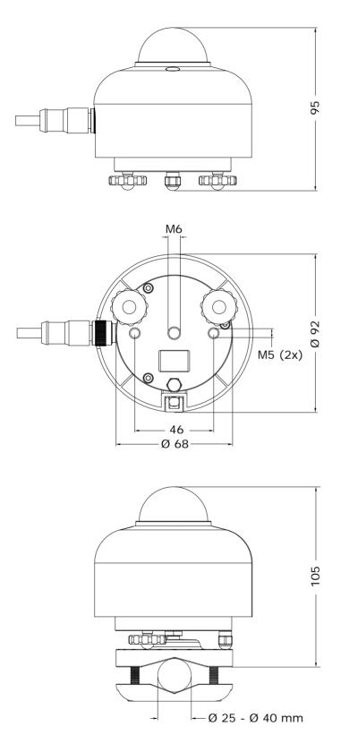
**Figure 3.2.1** Dimensions of SR30 in  $x \ 10^{-3}$  m. Mounts are optional
