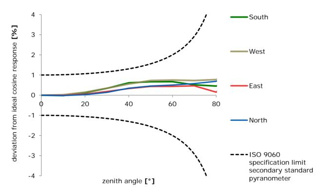
**Figure 2.0.3** *Directional response of an SR30 pyranometer of 4 azimuth angles, compared to secondary standard limits.*
