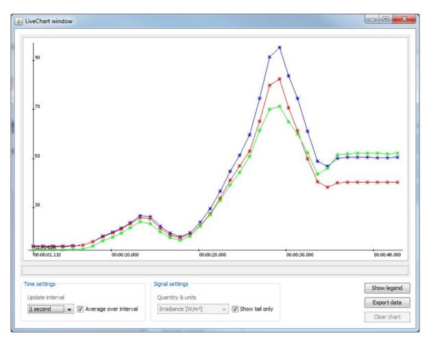
Figure 7.1.4.1 Example of an SR30 irradiance plot in the Sensor Manager
