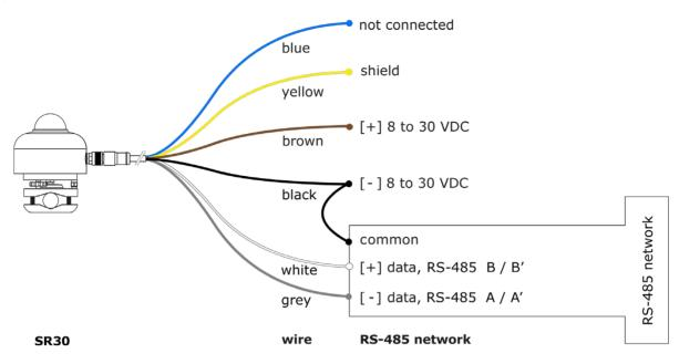
**Figure 6.7.2** Connection of SR30 to an RS-485 network. SR30 is powered by an external power supply of 8 to 30 VDC.
