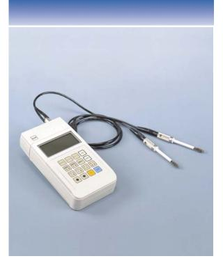
For building and waterproofing industries, moisture control in concrete and mortar is one of the most important factors. The model HI-500 proves to be an ideal moisture tester since it employs a dielectric constant principle which can search the average moisture content to a depth of up to 4 cm.
