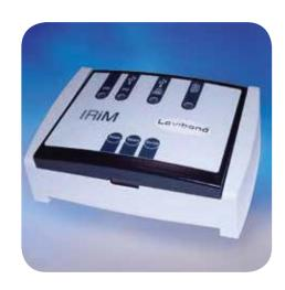
The IRiM (infrared interface modul) uses modern infrared technology to transmit measurement data from the MD 600 photometer to one of 3 optional interfaces. These interfaces can be used to connect to a PC, a USB printer<sup>1)</sup> or alternatively a serial printer<sup>2)</sup>. The interface which is selected is displayed by an LED function indicator. The user can switch between the interfaces using the "Select" button.
