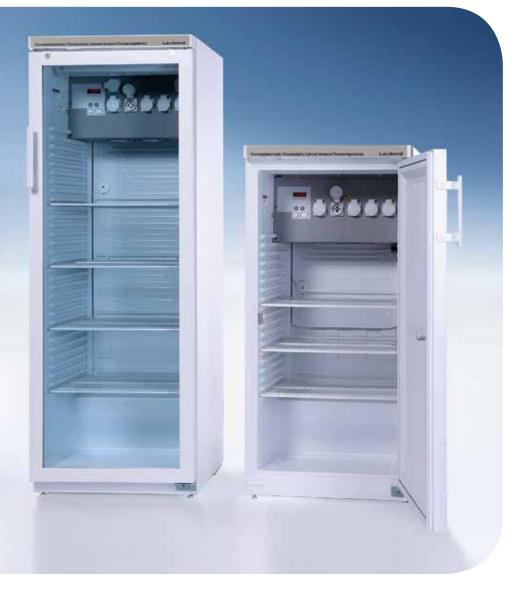
The TC series of thermostatically controlled cabinets is used for continuous temperature control over a range of 2 °C to 40 °C. This makes them ideal for a wide range of different applications in industrial and research laboratories.
