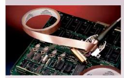
EMI-RFI copper tape shielding
