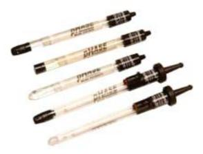
Fast - response stable to 0.01 pH within 30 Seconds with temperature change of 35C to 75C
