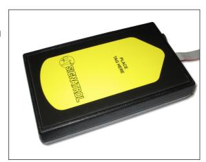
Communication is via a short range radio interface (300K Hz) which is provided by the SL150R Reader. The tag should be placed on the reader orientated as shown on the decal (Either side up).
