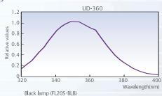
Black lamp (FL20S·BLB) Calibrated at irradiance of 320nm to 400nm in wavelength
