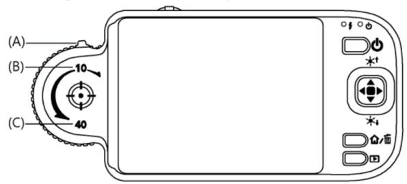
(2) Horizontal contact: there are two focus points (10x & 40x) in horizontal-contact observation, slightly tuning theblack indicator so that to get the clearest image quality
