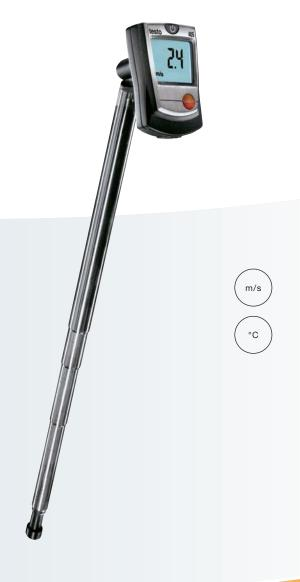
testo 405 is a thermal anemometer. It allows the precise measurement of air flow velocity, volume flow and temperature. With the extendable telescope (up to 300 mm), testo 405 is particularly suited for measuring the flow velocity in ducts. Thanks to the attachment included in delivery, the telescope can be optimally positioned in a duct.
