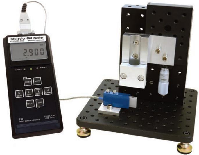
The PosiTector SHD Verifier and the included documents allow the user to certify the accuracy of PosiTector SHD Shore Hardness Durometers in-house.
