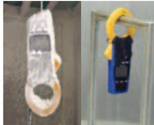
In the dustproof test, the clamp meter's enclosure is placed under reduced pressure and exposed to dust, and in the waterproof test, the instrument is sprayed with water from multiple directions in order to investigate how readily dust and water can enter.
