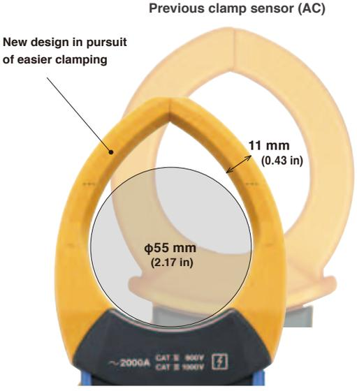
Narrowest width of jaw cross-section: 11 mm (0.43 in)
