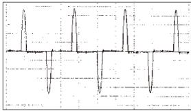
Current waveform from an inverter (primary side)
