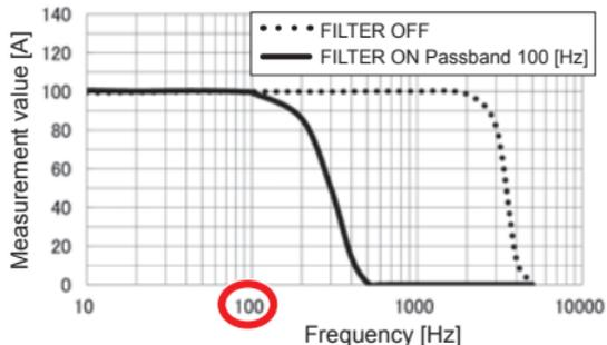
Turn off the filter function when performing measurement of power supply frequencies in excess of 100 Hz, for example on an aircraft or ship.
