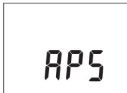
You can turn the display back on by pressing a key or by turning the rotary switch.
