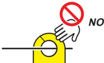
**Do not clamp around two wires.**
