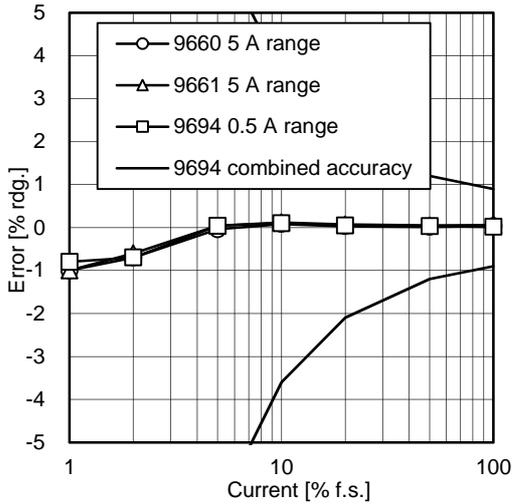
Fig. 11. Current Linearity Characteristics (50 Hz)
