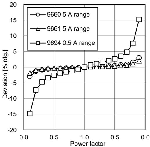
Fig. 13. Effects of Power Factor (50 Hz)
