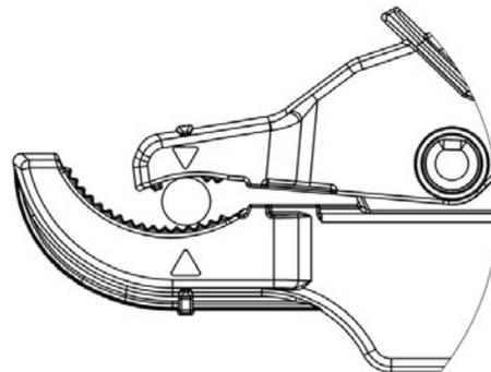
Fig. 6. When Clipping to a Cable With a Diameter of 6 mm
