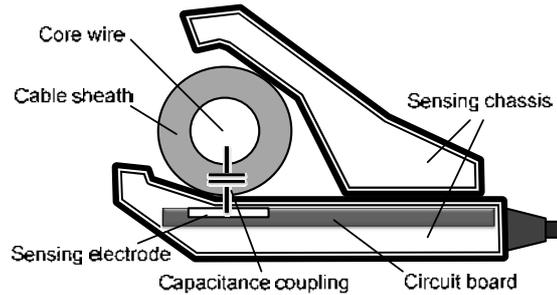
Fig. 1. PW9020 Electrode Design (Cross-sectional view)
