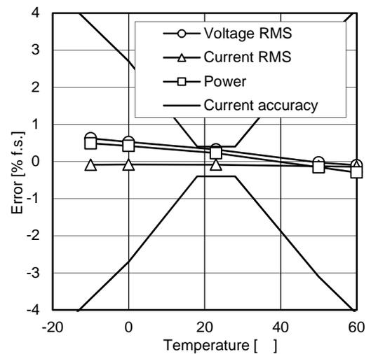
Fig. 14. Effects of Temperature (50 Hz)
