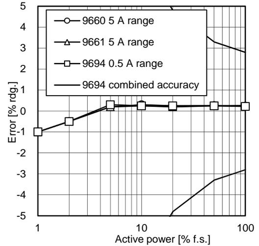
Fig. 12. Power Linearity Characteristics (50 Hz)
