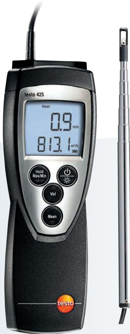
testo 425 is a compact anemometer with a fixed thermal flow velocity probe. The probe head has a diameter of 7.5 mm. With the extendable telescope (length max. 820 mm), the measuring instrument is suitable for flow velocity measurement in ducts. The testo 425 also measures extremely accurately in the low flow velocity range. The volume flow is directly shown in the display. For the purposes of volume flow calculation, the duct area can be
