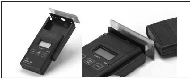
Figure 6. 718 Static Sensor charging plate in use.
