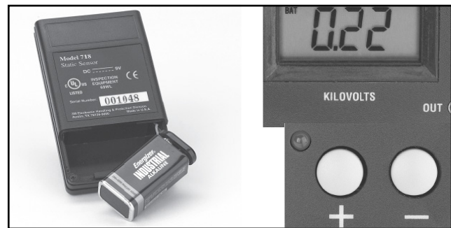
Figure 2. SCS 718 and 718A Battery Replacement and Indicators.
