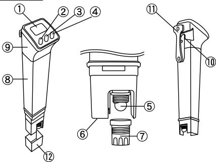
(1) LCD : Displays measurement readings or status of the unit.
