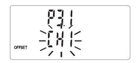
2) Use the ▲ or ▼ key to select the channel for which to set the offset, and then press the ENTER key. The ON or OFF setting display appears.
