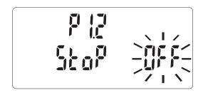
6) Use the [▲] or [▼] key to select "ON", and then press the [ENTER] key. The stop date and time setting display appears. When the preset stop is unnecessary, select "OFF". The preset logging setting screen is resumed.
