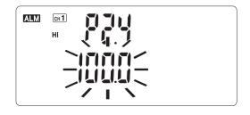
5) Use the  $[\blacktriangle]$  or  $[\blacktriangledown]$  key to change the alarm value, and then press the ENTER key to confirm.
