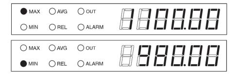
To reset the MAX or MIN value, press and hold the MAX/MIN key for at least two seconds while the maximum or minimum value is being displayed. The MAX and MIN lights, as well as the measured value, start flashing to indicate that the maximum and minimum values are reset.
