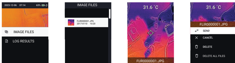
Figure 11.2 IMAGE FILES sub-menus. From left to right, press Menu at the IMAGE FILES menu, scroll to an image and press Menu, press Menu on an opened image and select from the available options.
