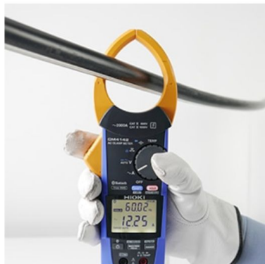
Position of the wire is in the center of the clamp (recommended)
