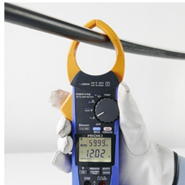
Position of the wire is out of the center of the clamp (discouraged)
